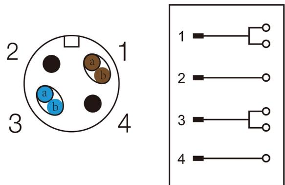
Pins 1 and 3 are power bits, which can be connected to the power cords of the two cables a and b respectively.
