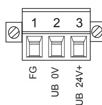
Note : UB is the module power supply
